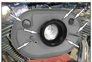
9. Install the two provided standoffs onto the filter back plate, then install the filter back plate onto the throttle body and secure first with the throttle body bolts and then with the breather bolts.
