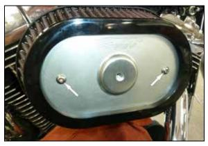
10. Place the K&N® filter on the back plate and attach with the remaining button head screws. NOTE: Apply one drop of provided thread locker to each screw.
