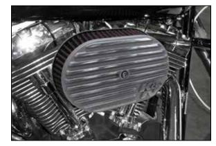
11. Attach cover plate with provided socket head Allen screw.
