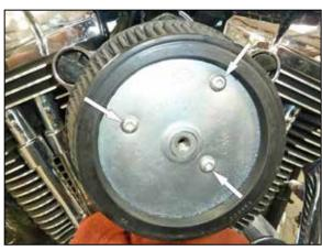
3. Remove the remove the three Torx screws that attach the air filter.
