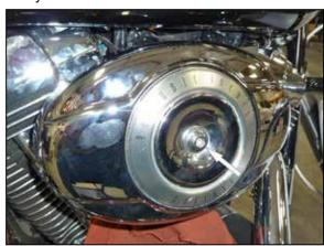
2. Remove the Allen screw that attaches the air filter cover.
