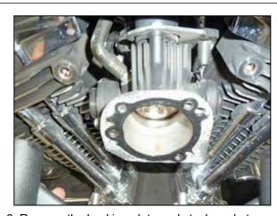
6. Remove the backing plate and stock gasket. NOTE: K&N Engineering, Inc. recommends that customers do not discard the factory air intake components.
