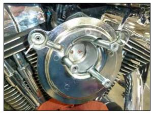
5. Remove the two rubber vent adapters from the vent bolts and then remove the two vent bolts.
