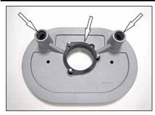
8. Install the remaining two O rings and the two filter spacers onto the front of the K&N® back plate as shown using the provided hardware.
